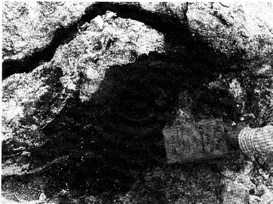
Figure 1. A small cave filled with interbedded sand and clay on west quarry wall at elevation of 760-770 feet amsl
